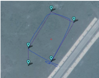
Figure 3. Blue line – real trajectory/Purple line – requested trajectory [21]
