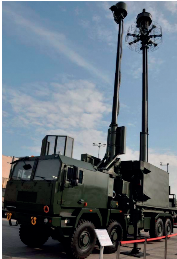
Figure 6. PIT-RADWAR's PET-PCL prototype radar [5]
