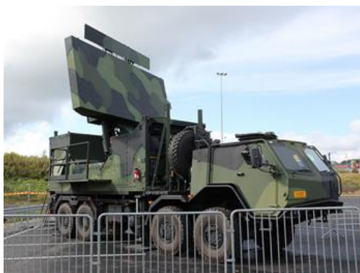
Figure10. Ground Master 403 radar [21]
