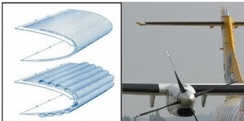
Figure 14. Pneumatic de-icing system [35]
