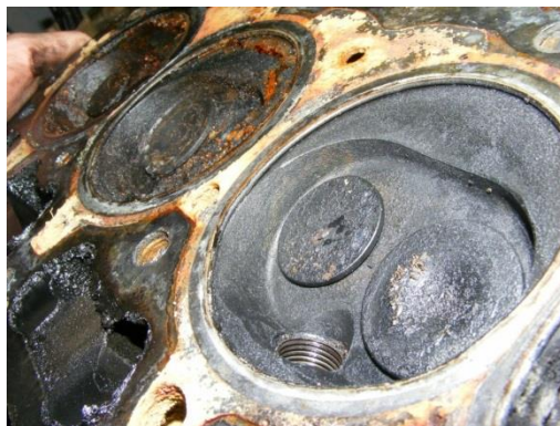
Fig. 6. Corrosion on the cylinder head of a combustion engine
