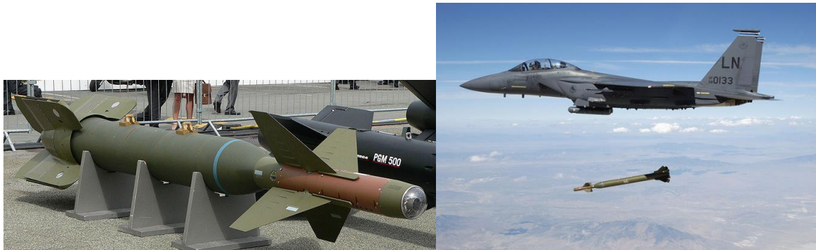
Fig. 3. GBU-28 laser-guided bomb, and its release from an F-15 of the U.S. Air Force 12
