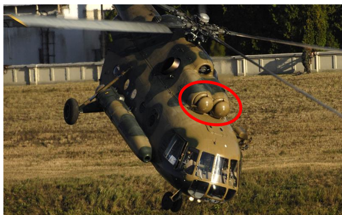
Fig. 5. PZU dust separator on Mi-17 transport helicopter
