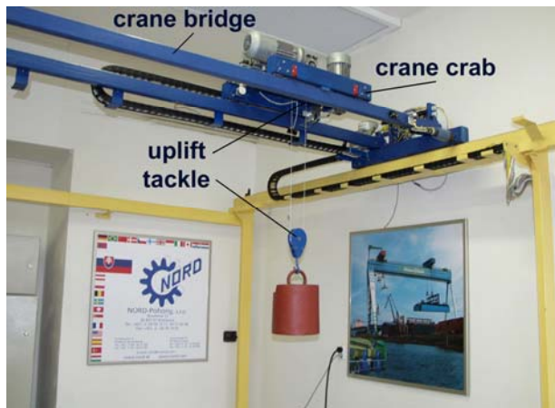
Figure 14 Experimental bridge crane
