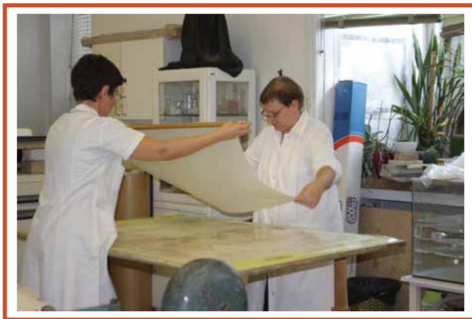
During paper mounting, the Japanese paper soaked in starch was put together of many parts.
