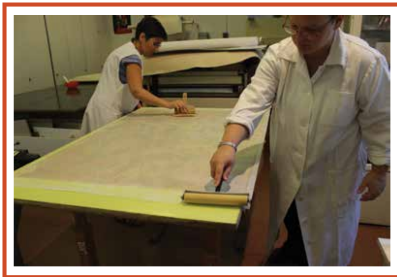
The paper mounting glue was smoothed by a paint roller and a Japanese paintbrush
