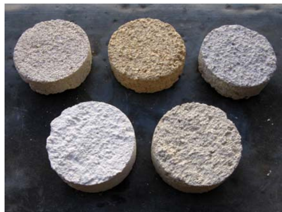
Fig. 9.: Color variation of lime mortar samples made with different sands of the project
